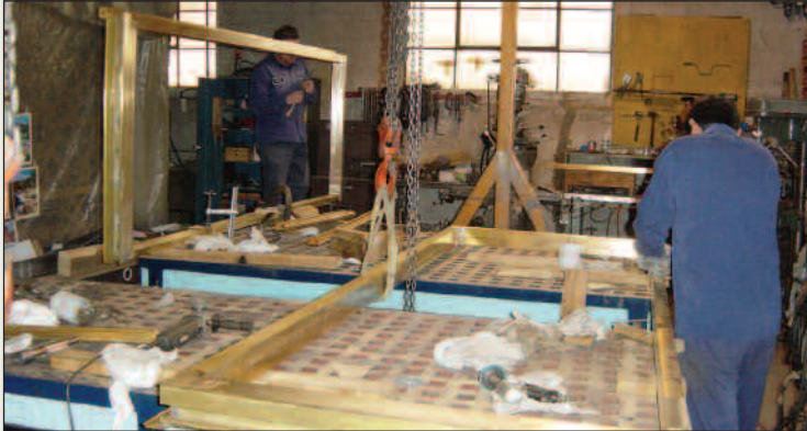
TOP: The door frames are assembled in the shop.
